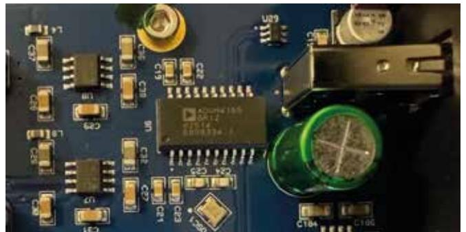
Metronome opted to forget all other digital audio interfaces, instead focusing on optimizing the USB output with isolation, reclocking, and Linux ALSA driver optimizations. The company suggests using a USB to S/PDIF convert for those who need support for such interfaces.
