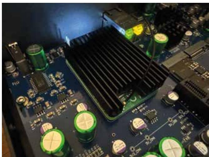
Left of the Compute Module 4 in the image, one can see a vertical USB port and an ADuM4165 digital isolator, providing galvanic isolation and clock regeneration to, “eliminate ground loops, reduce jitter, and ensure pristine signal integrity to any connected DAC.” Metronome nicely lists this chip in the DSAS Technical Guide, that I should’ve read before searching the internet for chip part numbers and features. This isolated US interface supports audio up through DSD512 and PCM 384 kHz.
