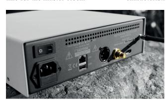
Additionally, data transfer occurs exclusively in a unidirectional mode. This gives I2S a reputation as a superior connection option in terms of sound quality, thanks to its reduced sensitivity to jitter. However, the main drawback of I2S lies in the lack of a standardized connector type. The Métronome DSS 2 uses the HDMI format for I2S, as, according to the manufacturer, this connection offers excellent electrical properties for this purpose.
