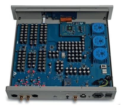
The original design of the **DAC** visually showcases a robust setup of three encapsulated toroidal transformers, complemented by an impressive array of capacitors dedicated to six independent regulation lines.
