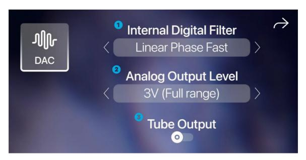
My filter choice was "Linear Phase Fast". My Tube Output was switched on for most of the duration. Other filter choices include Linear Phase Slow, Minimum Phase Fast, Minimum Phase Slow, Apodizing Fast, Minimum Phase, Brick Wall, and Corr. Minimum Phase Fast.
