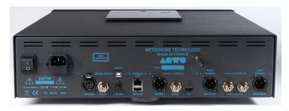
The rear of the unit has all connectivity covered. USB asynchronous type B, S/P DIF 75 Ohms RCA, AES-EBU 110 Ohms XLR, I<sup>2</sup>S HDMI proprietary, Toslink, Unbalanced RCA x2, Balanced XLR x2, WiFi antenna connection (the antenna was not provided with the review unit), LAN socket and standard IEC power socket with rocker on/off switch.
