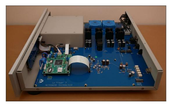
Le DAC then packs 2 x 5VA and 2 x 12.5VA transformers plus 158 of the same caps we saw in Le Player 3+ plus 4 x SCR MTPA 02 caps, the big white cubes which Nagra are fond of as well.
