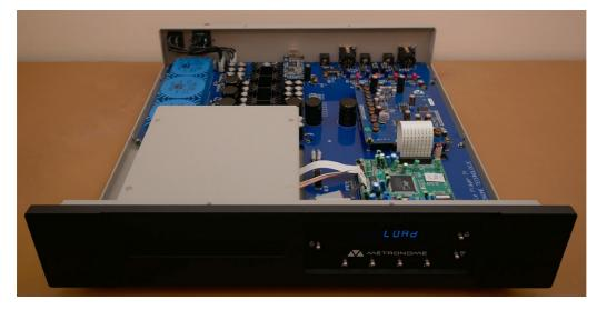
... packs 1 x 5VA and 2 x 7.5VA transformers plus 40 smaller capacitors. The encased transport mechanism is obviously shared with the pure transport.
