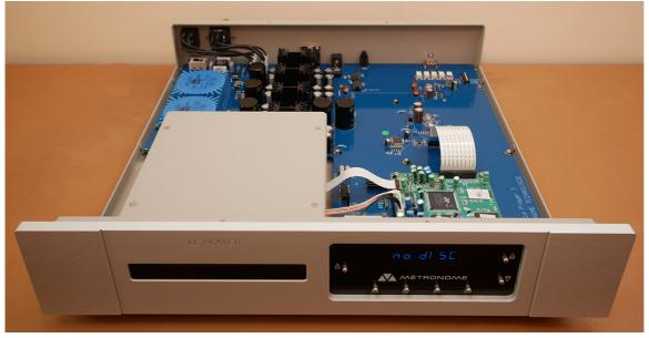
... gets 2 x 7.5VA transformers plus the same four voltage regulators with finned heat sinks as the CDP/DAC.
