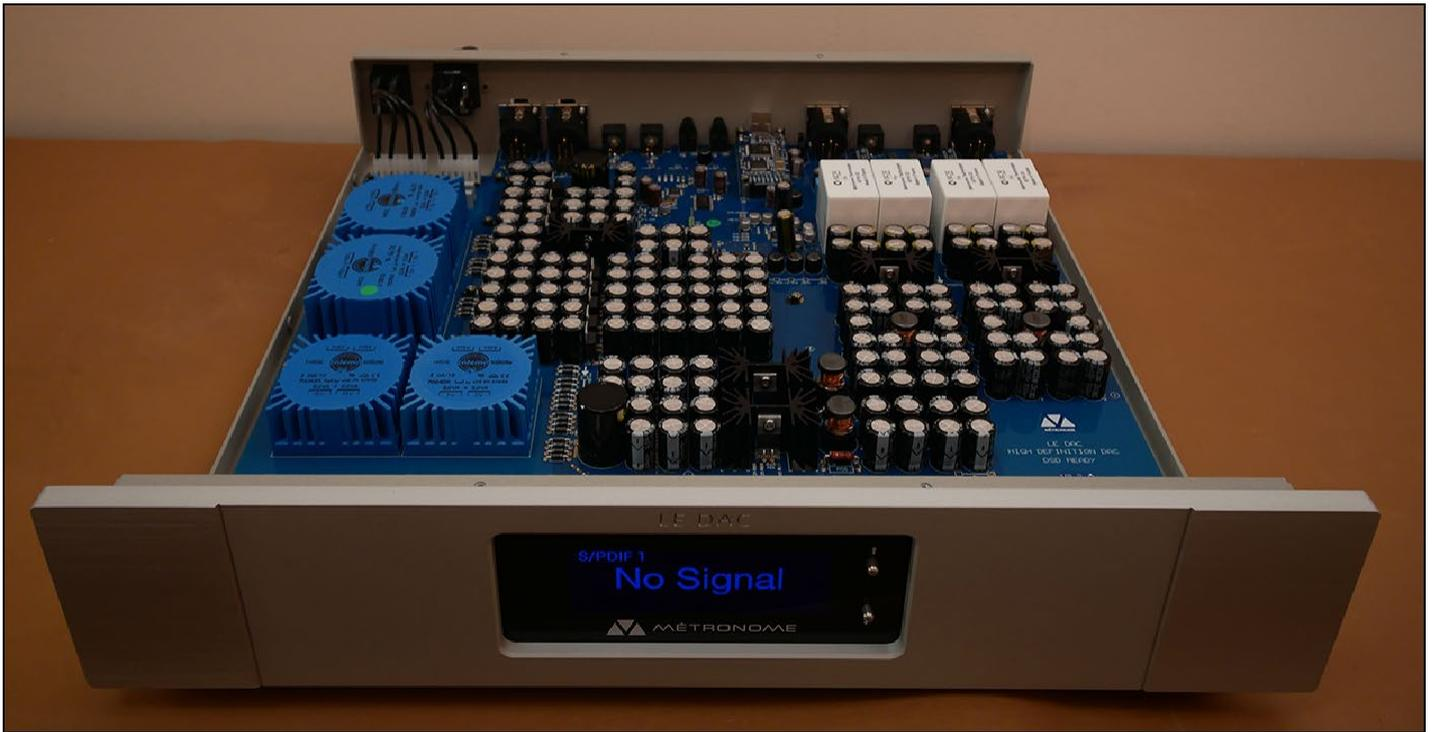
In short, the separates get *twice* the number of transformers and *wildly* more capacitance/filtering. On the latter score, Le DAC actually looks like a Denafrips. It sports the same phalanx of massively paralleled capacitor warriors
