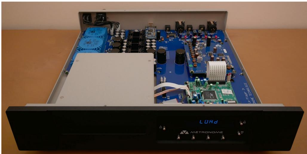
... packs 1 x 5VA and 2 x 7.5VA transformers plus 40 smaller capacitors. The encased transport mechanism is obviously shared with the pure transport.
